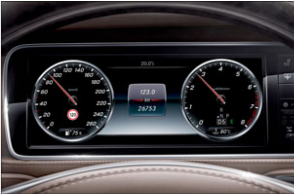
Traffic Sign Assist can recognise speed limit signs and show the speed limit on the display.
