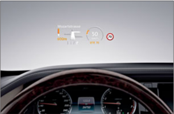
The head-up display posts information directly within the driver's field of vision.
