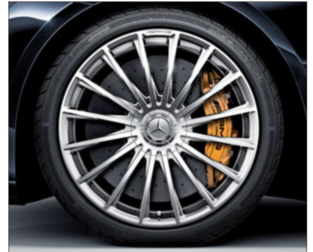
The standard-fit AMG 20-inch multi-spoke forged wheels with optional AMG ceramic high-performance composite brake system.
