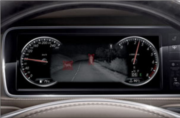
Night View Assist Plus highlights any people it has recognised and helps the drivers to react quicker to dangers by night.
