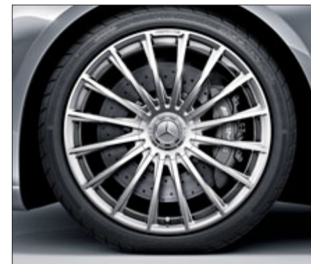
AMG multi-spoke forged wheels, with ceramic high-gloss polish finish, with 255/40 R 20 front and 285/35 R 20 rear tyres (only for S 65 AMG, Code 696).
